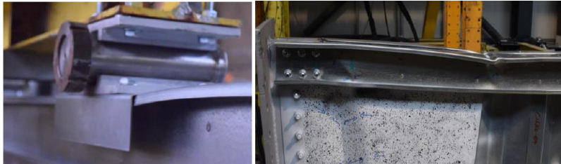
Figure 16: Local deformations under the load application point.
