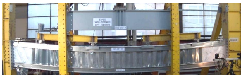
Figure 11: CWB-SW1 beam – global deformation during the testing.
