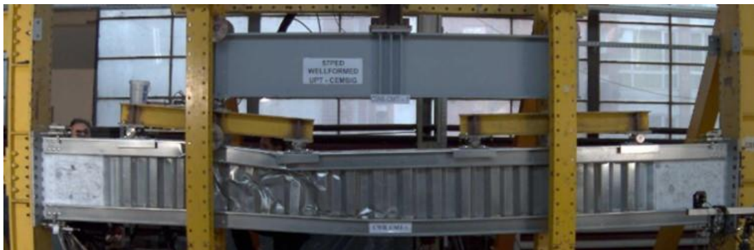
Figure 7: Deformed shape of CWB-CMT1
