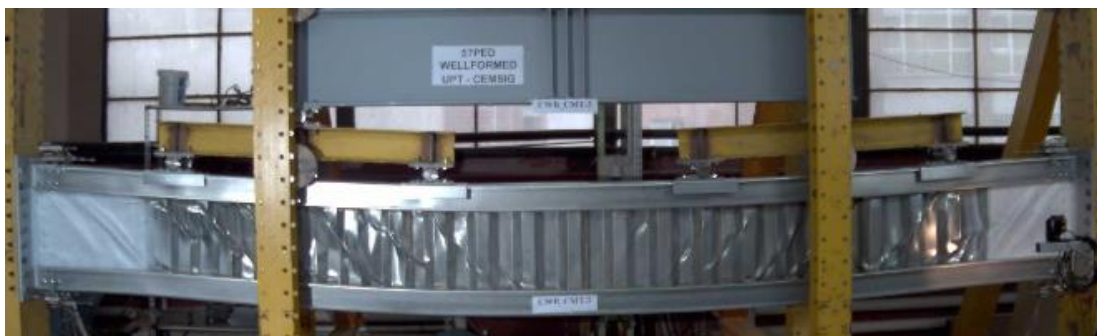
Figure 12: Deformed shape of CWB-CMT3
