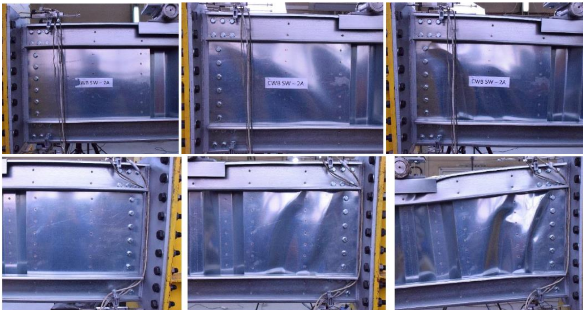
Figure 20: Development of the shear buckling at the end panels for CWB SW-2 beam.
