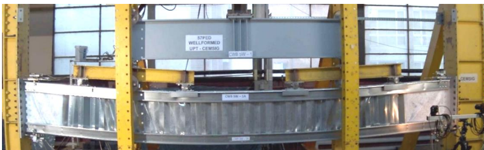
Figure 15: CWB-SW1 beam – global deformation during the testing.
