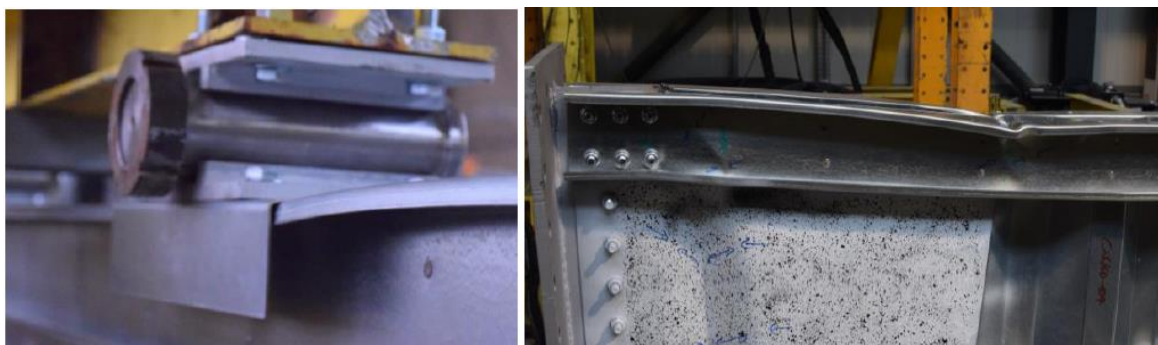
Figure 24: Local deformations under the load application point.
