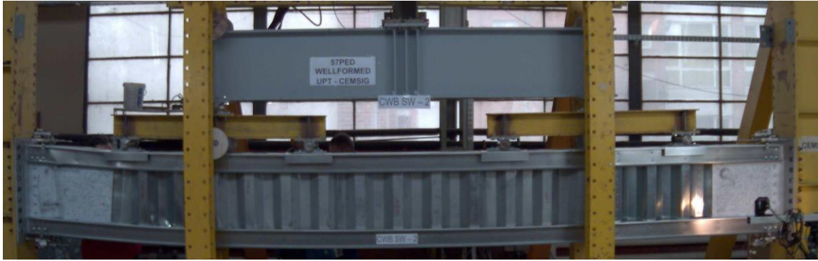
Figure 19: CWB SW-2 beam – global deformation during the testing.
