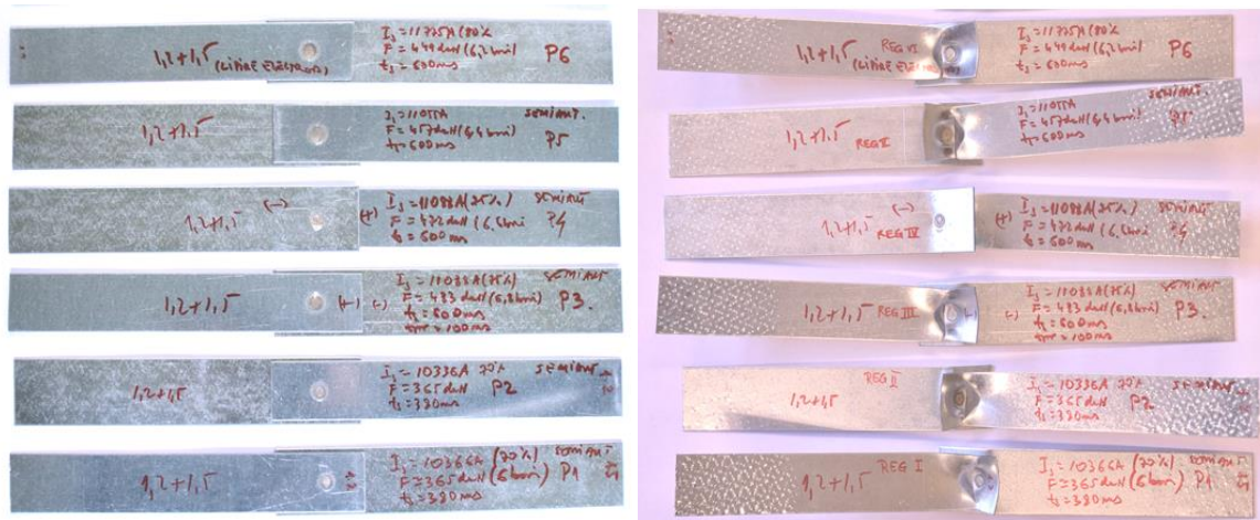
Figure 3: Specimens SW-1.2-1.5 before and after testing, using different welding regimes.
