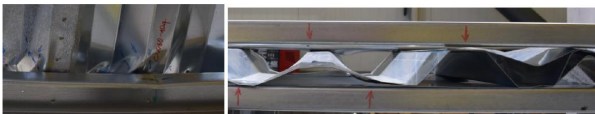
Figure 21: Distortion of the web corrugation of the CWB SW-2 beam.
