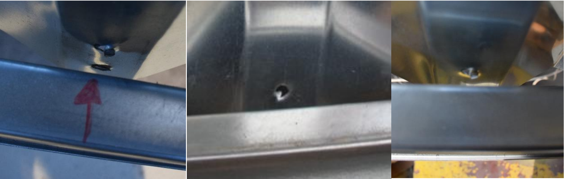
Spot welding failure between the web and the flange
