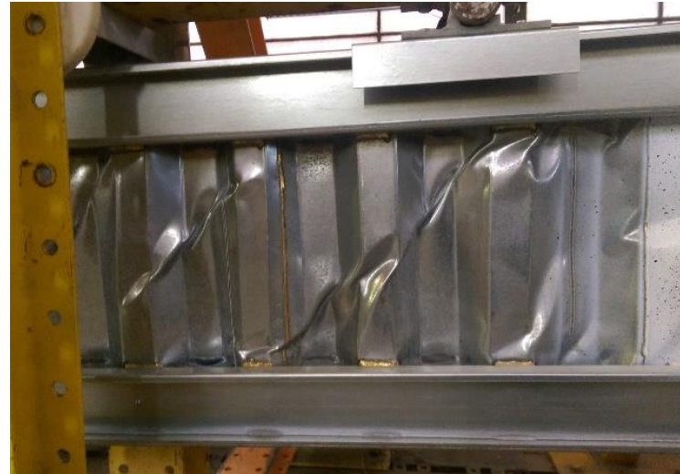
Shear buckling of the web corrugation
