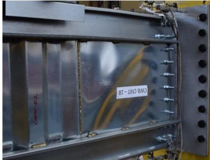
Development of the buckling of the end shear panels
