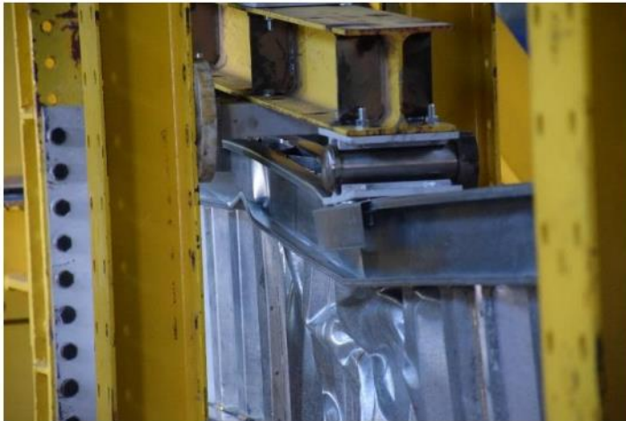
Shear buckling of the web corrugation
