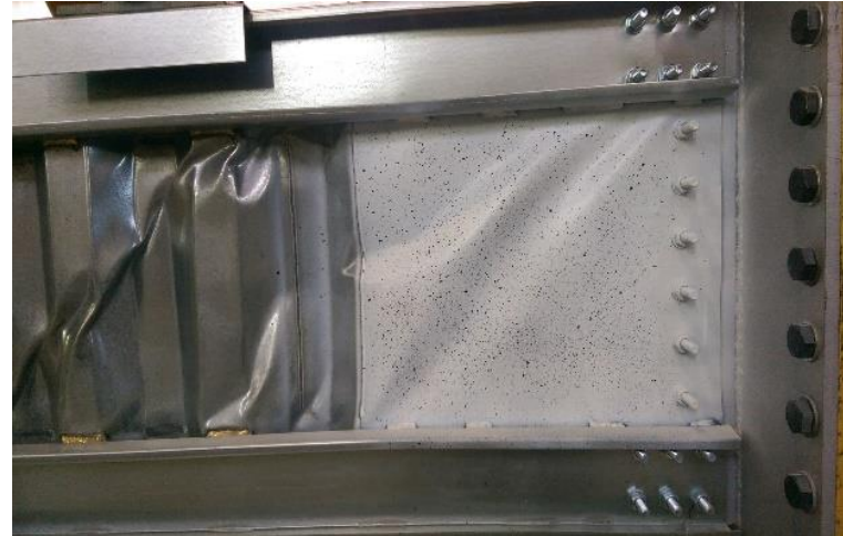
Development of the buckling of the end shear panels
