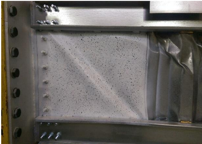
Development of the buckling of the end shear panels
