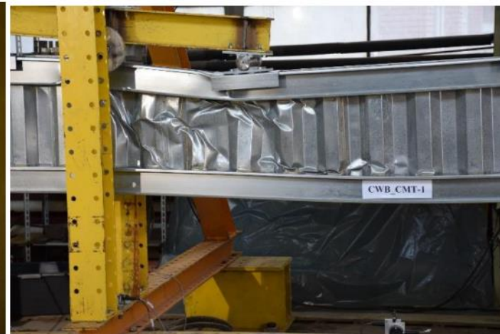
Shear buckling of the web corrugation
