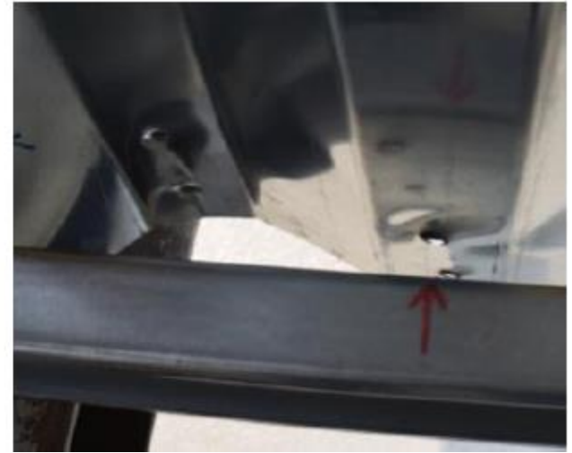
Spot welding failure between the web and the flange
