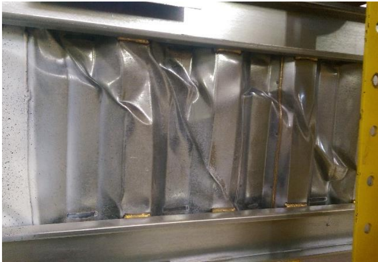
Shear buckling of the web corrugation
