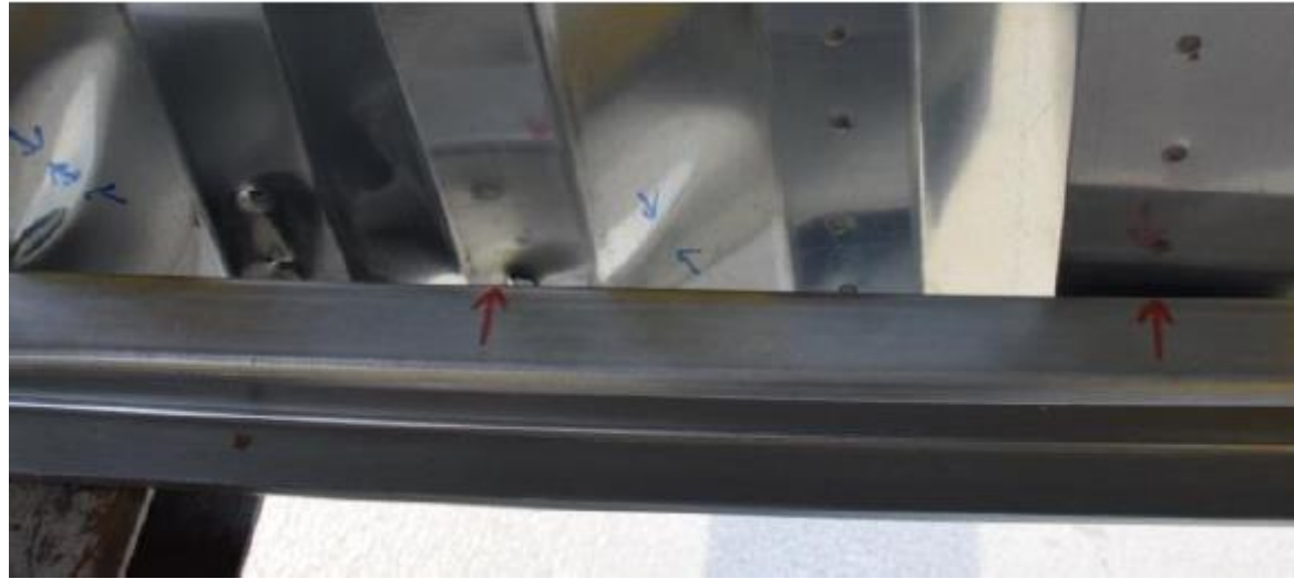
Spot welding failure between the web and the flange
