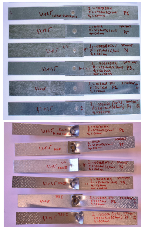
Fig. 6 – Specimens SW-1.2-1.5 before and after testing, using different welding regimes.
