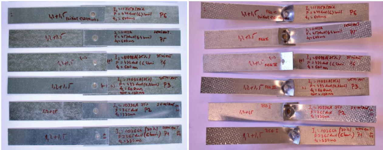
Fig. 6. Specimens SW-1.2-1.5 before and after testing, using different welding regimes
