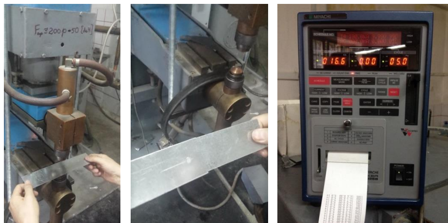
Figure 2. Spot welding process
