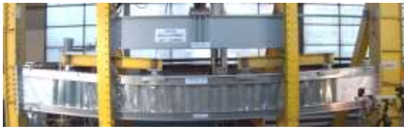
Fig. 13. CWB-SW1 beam – global deformation during the testing.
