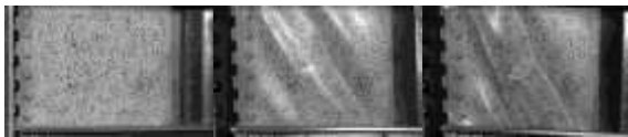
Fig. 14. Development of the shear buckling at the end panels for CWB SW-1 beam.
