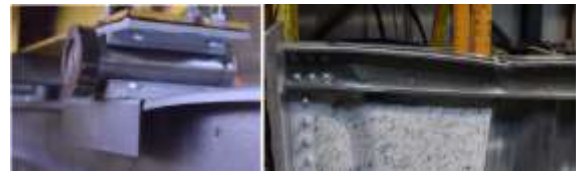
Fig. 18. Local deformations under the load application point.
