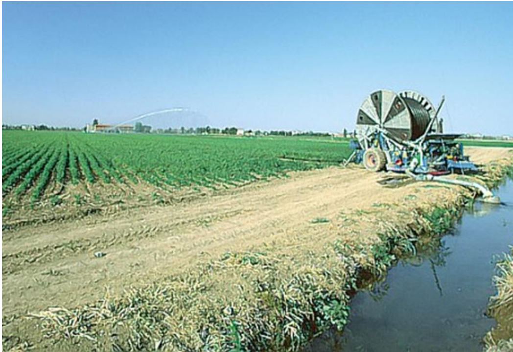
Figure 11. Overview of the drum and hose irrigation system in operation
