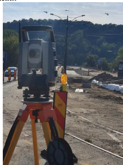
Figura 4. Trimble S7 total station
