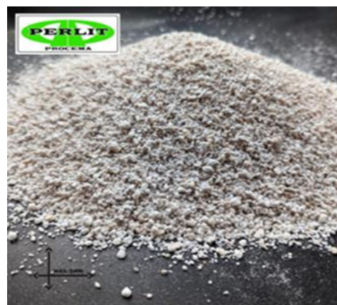
Figure 5. Granular perlite used in concrete [1]
